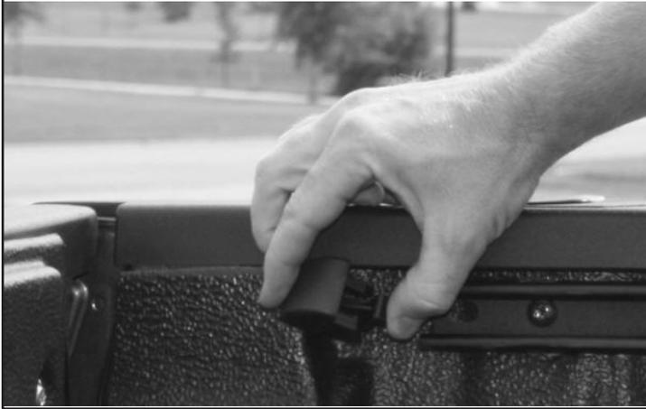
**2** Remove tie downs: If tie downs are installed remove them from the cargo rail.
