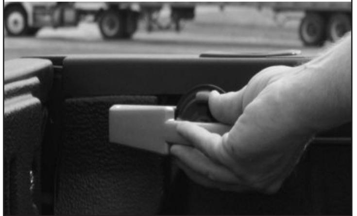
**3** Install clamps: Slide the female side of clamp into the cargo rail. See step five to correctly arrange the order of the clamps and tie downs.
